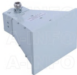
LB-2080-NFSPO Broadband Horn Antenna 2-8GHz 12dB Gain N Type Female
